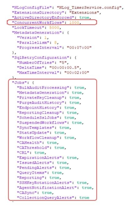
Figure 406: Appsettings.json File for TimerService Settings
