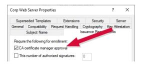
Figure 127: Certificate Template Requiring Manager Approval
